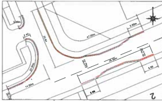
Road Marking : Location 3 North Peffer Place junction with Peffer Place. Scale 1:250
