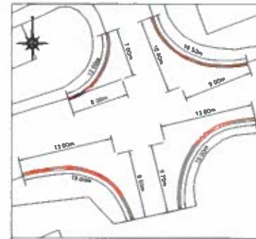
Road Marking : Location 6 Access roads on Peffer Place approx 126.00 metres from North Peffer Place. Scale 1:250
