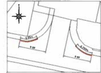
Road Marking : Location 7 Access road at Harewood Road at Industrial Units. Scale 1:250
